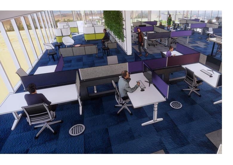
Enhanced HVAC to purify contaminated air particles are vital in the open-plan office. There are many potentially effective solutions; here, we chose one that's common in Europe and Asia but lesser known in the U.S.: underfloor air distribution paired with an overhead plenum, with registers positioned over occupants' desks, that sucks up impurities. To promote wellbeing, ceiling elements with flexible louvers allow additional fresh-air intake as well as UV-light access.
